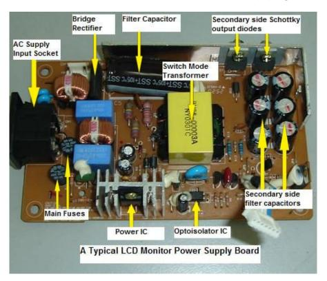
Troubleshooting linear power supply was quite easy as compare to switch mode power supplies (SMPS). AC voltage enters to the primary side of linear transformer and then converted the AC into a lower or higher AC voltage depending on the secondary winding. The output AC voltage is then rectified and filtered by a diode and capacitors to produce a clean DC voltage.
