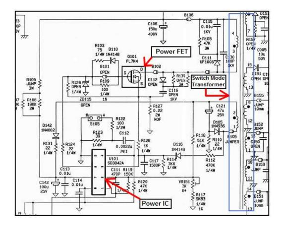
Once the PWM IC received the voltage it will output a signal to drive the transistor (or FET) and produces a changing in magnetic field in the transformer primary winding. The changing magnetic field induces voltage in the secondary windings.
