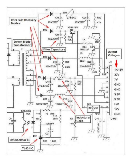
The output from the B+ voltage supply is then connected, through a "feedback" loop (which consist of optoisolator ic and an error amplifier TL431 IC), back to the PWM IC. When the voltage from the B+ supply rises or drop a bit, the PWM IC will act to correct the output.
